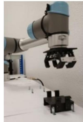
Test bench for the validation phase of an IFMIF-DONES remote handling robot
